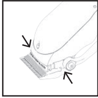
PERIODICALLY OIL HEEL OF BLADE
